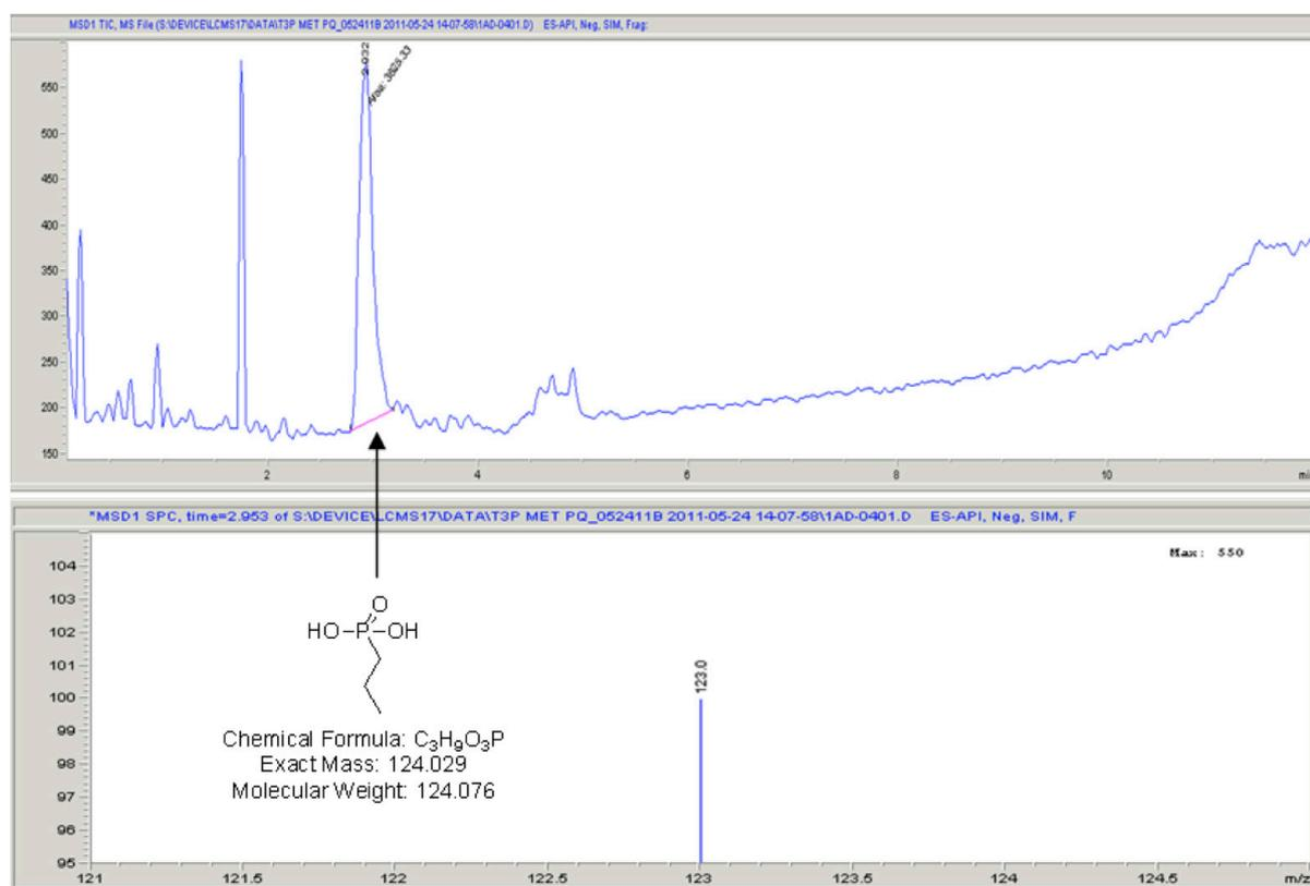
Figure 8. Representative Chromatogram of Propyl Phosphoric Acids by Reversed Phase LC-MS with Total Ion Current (TIC) Signal and Corresponding Mass Spectrum
