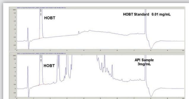
**Figure 4. Representative Chromatogram of HOBt by Reversed Phase HPLC with UV Detection**
