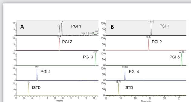
**Figure 4. Chromatograms of 4 ng/mL of PGIs spiked into 4mg/mL of API. (A) The data was acquired on QqQ-MS instrument. (B) The data was acquired on high-resolution MS instrument.**
