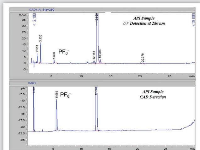
**Figure 5. Representative Chromatogram of PF<sub>6</sub><sup>-</sup> by Reversed Phase HPLC with CAD and UV Detection Note that PF<sub>6</sub><sup>-</sup> is not detected by UV.**
