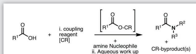
Figure 1. Schematic illustrating the generation of an amide bond in the final product and a byproduct using a coupling reagent (CR).
