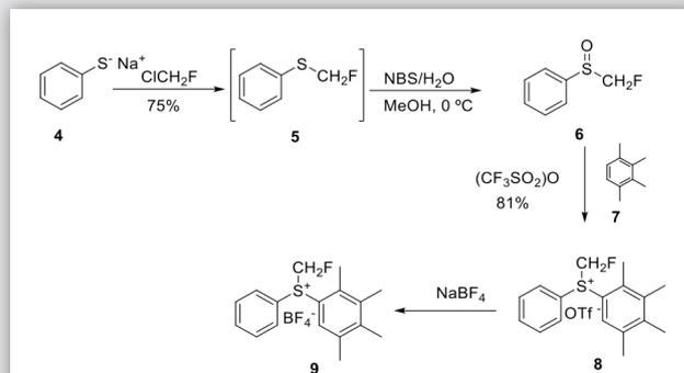
**Scheme 1.** Synthesis of S-monofluoromethyl-S-phenyl-2,3,4,5-tetramethylphenylsulfonium tetrafluoroborate salt (**9**).
