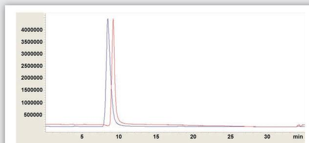
**Figure 3. Representative Chromatograms of EDC (red) and its Urea Byproduct (blue) by Reversed Phase LC-MS with Single Ion Monitoring (SIM) Signals**
