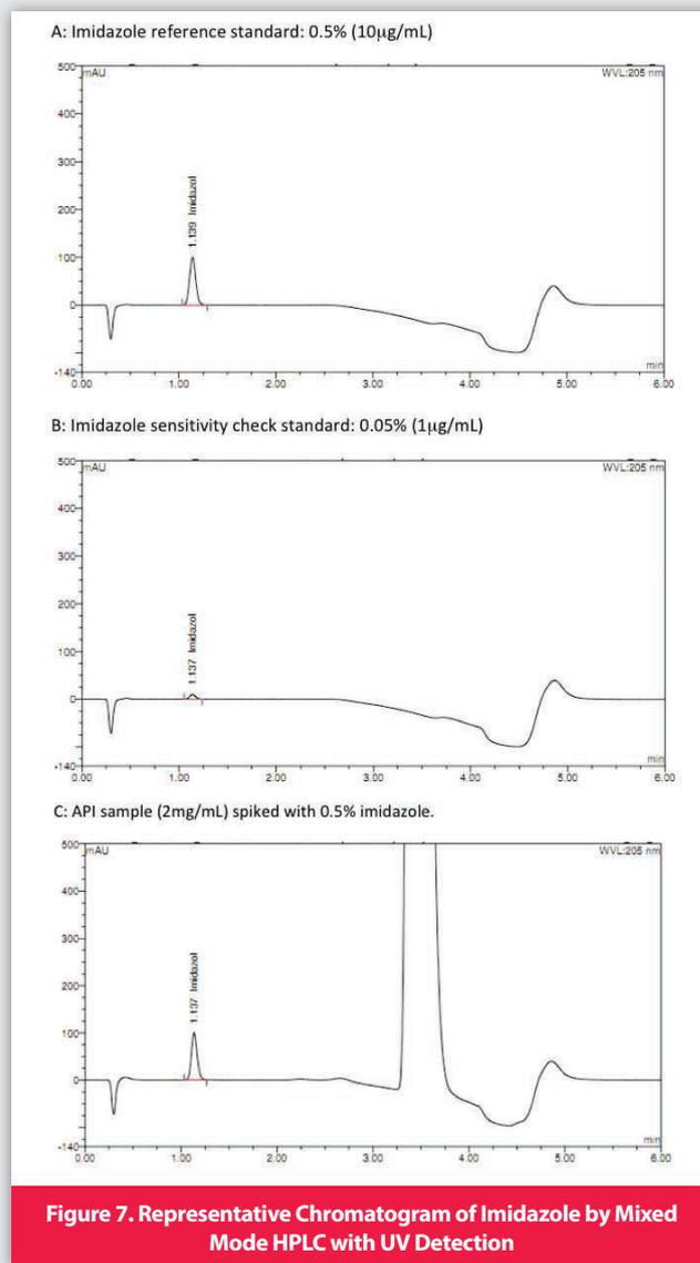
Figure 7. Representative Chromatogram of Imidazole by Mixed Mode HPLC with UV Detection
