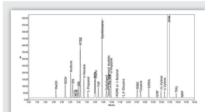
**Figure 6. Representative Chromatogram of TMU by Head Space-GC with FID Detection [12] Showing Other Common Solvents in a Generic Method for Residual Solvent Analysis**
